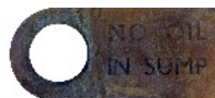
Printed on cardboard labels attached to the engine were warnings that the engine had been preserved and certain precautions were required before starting it.
